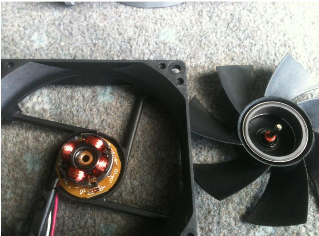
12. Find something blunt and larger than the brass sleeve bearing (like a cross head screwdriver) and with the fan on a flat surface push the bearing down hard.
