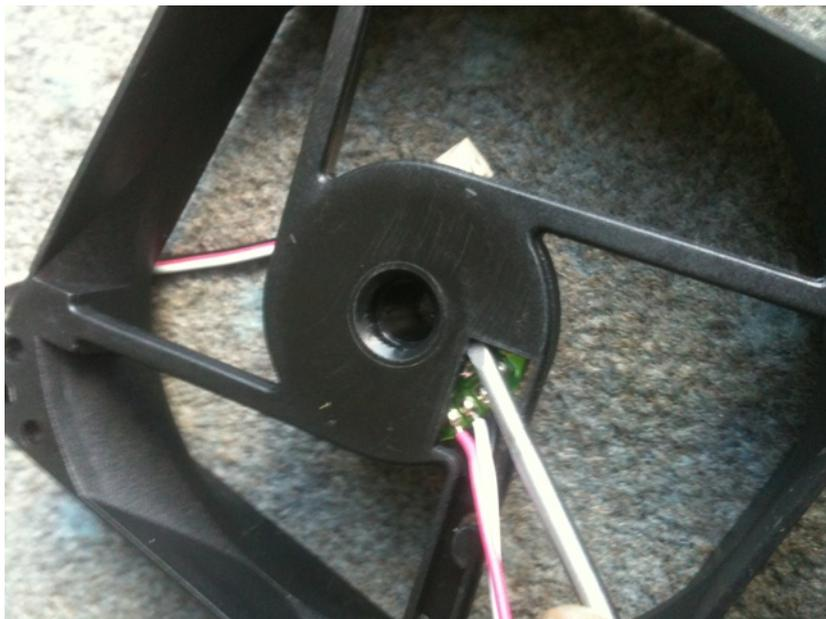
16. Alternate step 15 with gently working the board loose from the front as shown. Do NOT try to pull the top coil part of the stator as you can easily break it....just be patient until the board starts to move up the shaft.
