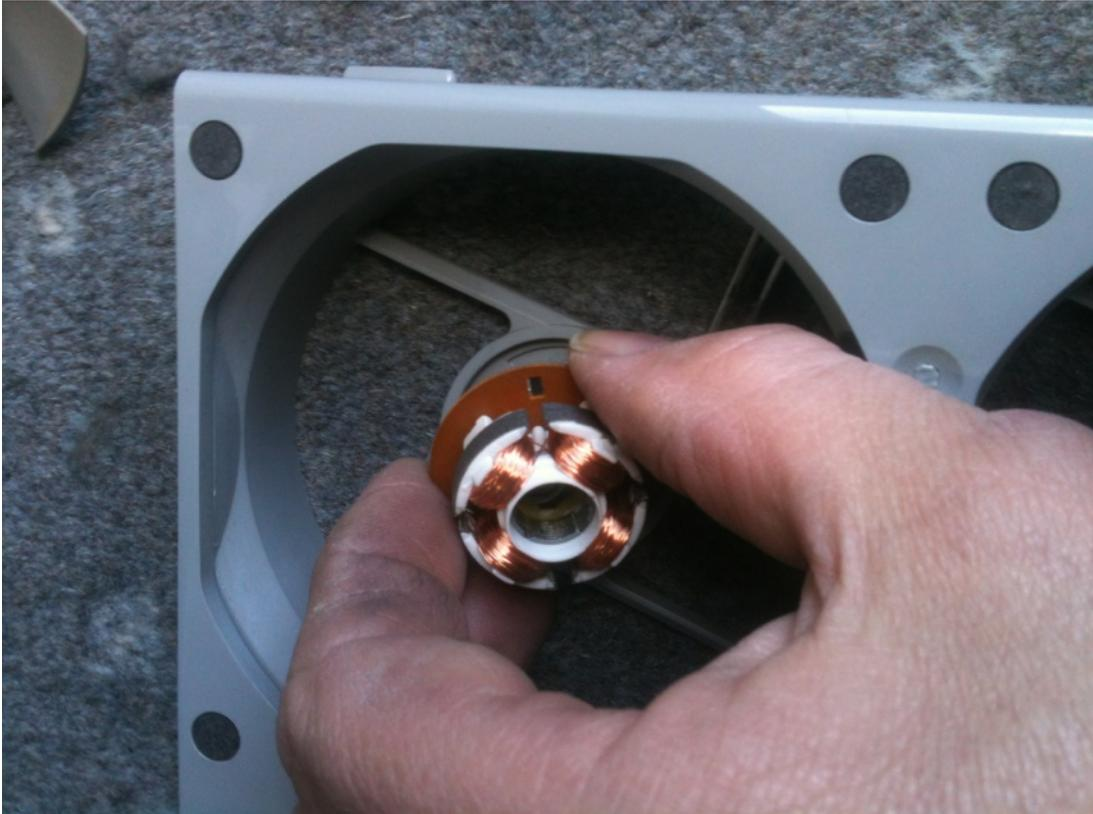
You now have this. The stators removed from the frame and you can see the top bearing in the shafts (don't worry if they fall out - just place them back in they are a loose fit) and there are also separate bearings underneath.
