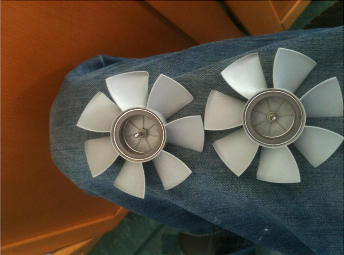
26. Fit the rotors back in place and then re-fit the white plastic clips. The original ones or the Zalman ones will fit. You can use your multitool to push it back onto the rotor shaft.
