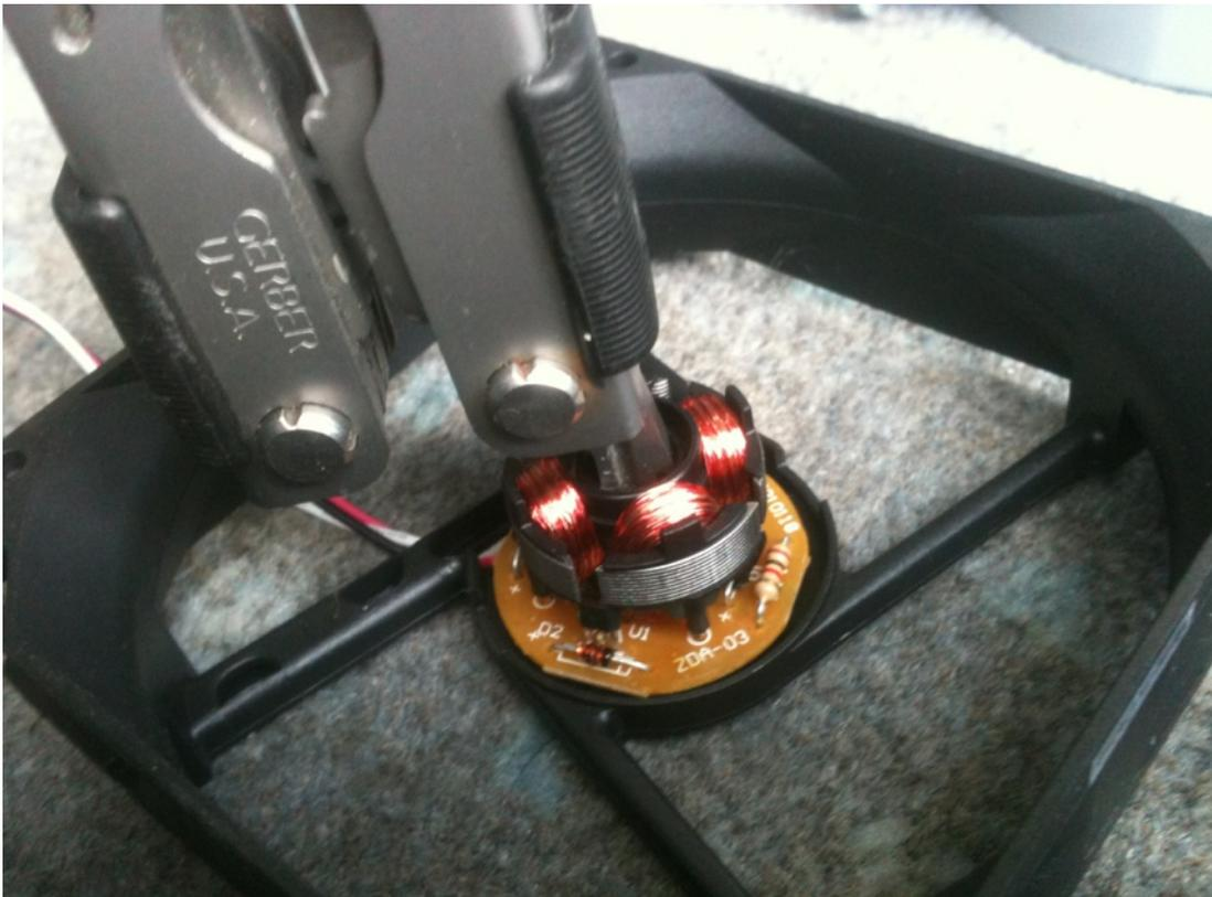
14. When the bearing has slipped through you can pull it out from underneath.
