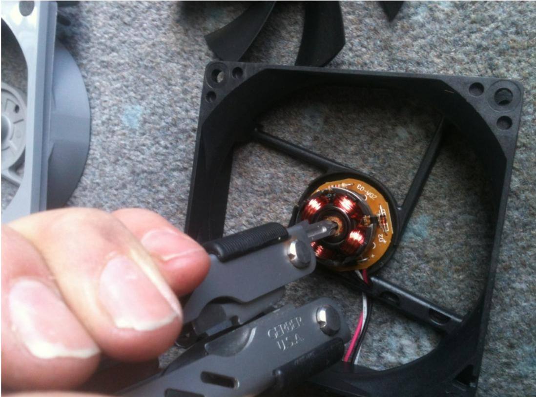
13. The idea is to push the sleeve out through the bottom of the fan frame as shown.
