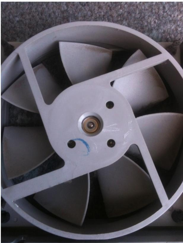
3. Here is a close look. You can see the rotor spindle, that is held on by a little white plastic circular clip and underneath that is a bearing.
