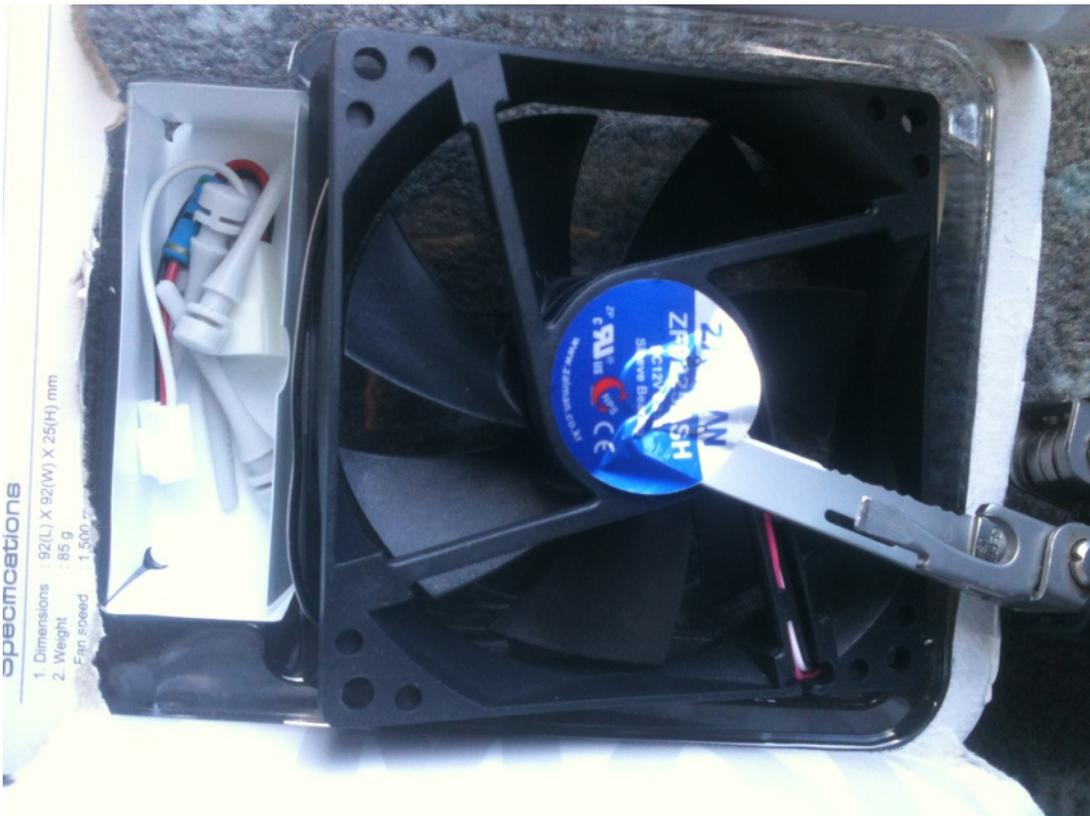
9. Remove the sticker and then carefully pull the wiring from the retaining clips in the frame.
