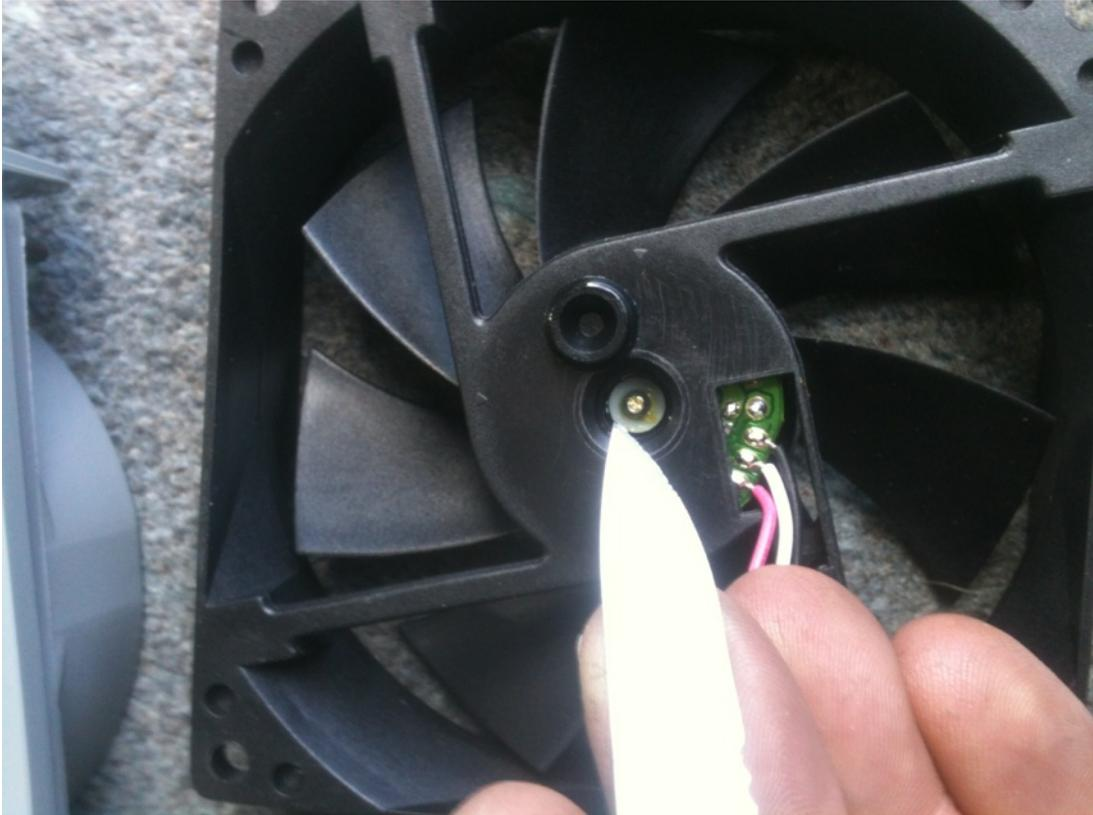
11. Rotor now comes off and can be thrown away. Notice though the bearing here is a solid brass sleeve. Your next job is to remove it without damaging the stator board.
