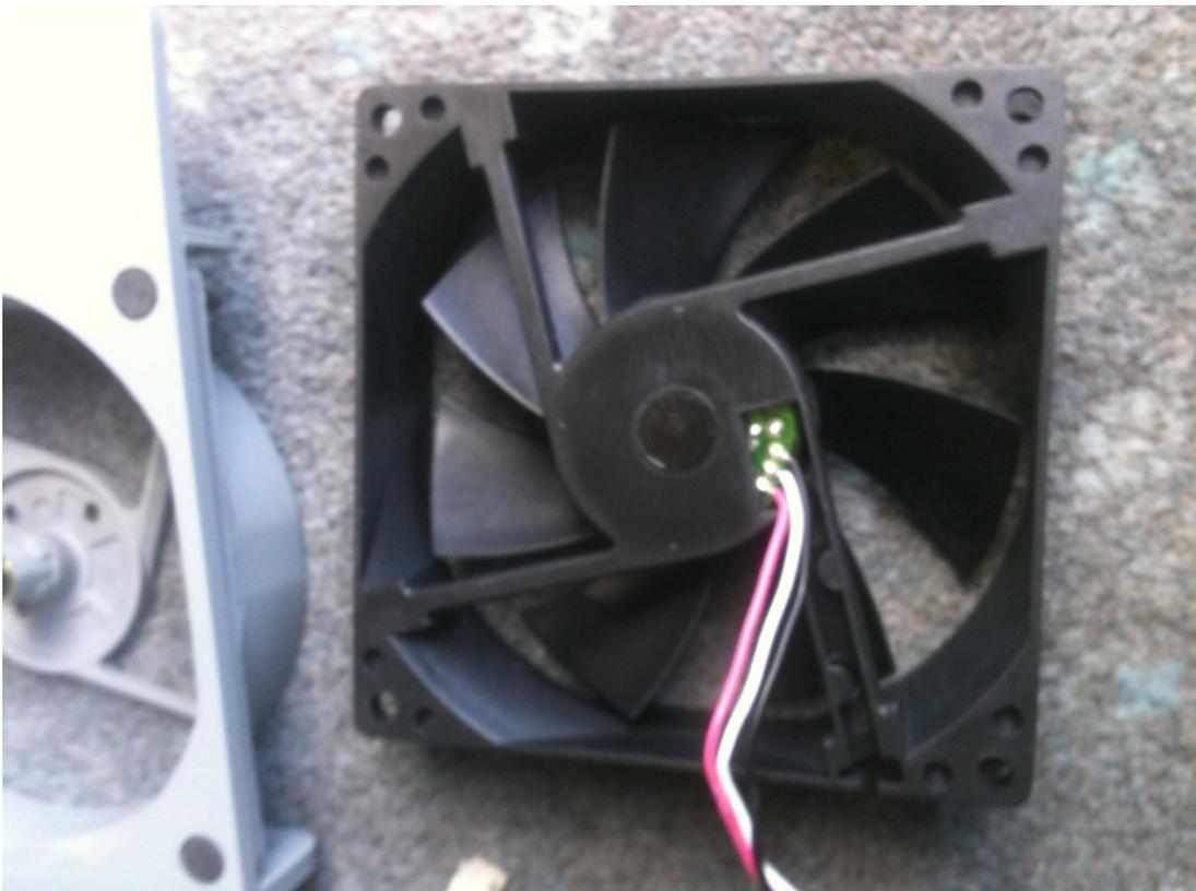
10. Remove the rubber cap (keep it you can re-use it) and in the same way as with the G5 fans prise off the little circular white plastic clip.
