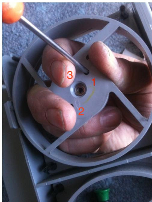
8. When the stator board starts to move you can use your fingers from the other side to pull it off the plastic shaft.
