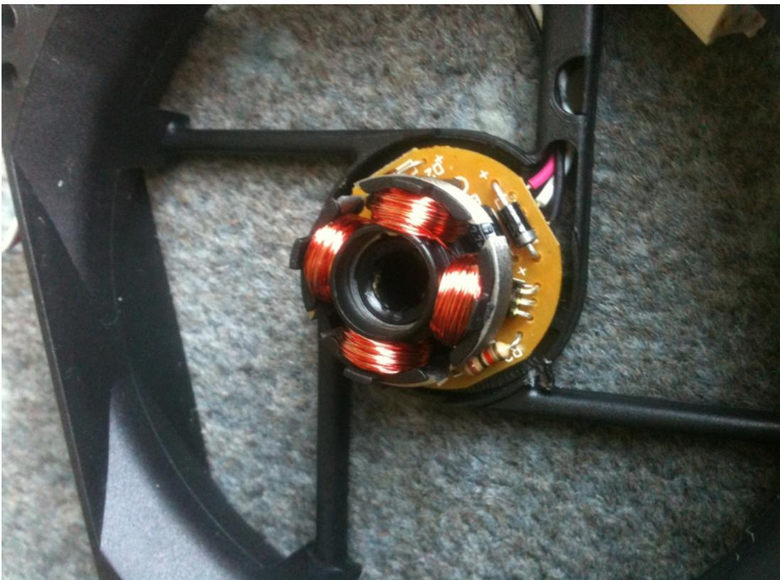
17. Once the board is freely moving off the shaft you can pull it clear and then pull the wiring from the frame.
