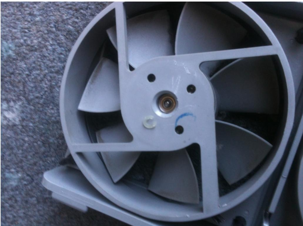
6. The rotors now just can fall off. Basically all fans have a the same inner rotor construction, it is a circular permanent magnet. They rotate when current is passed in the coils of the stator. Notice the springs on the rotor shaft. Don't lose them.
