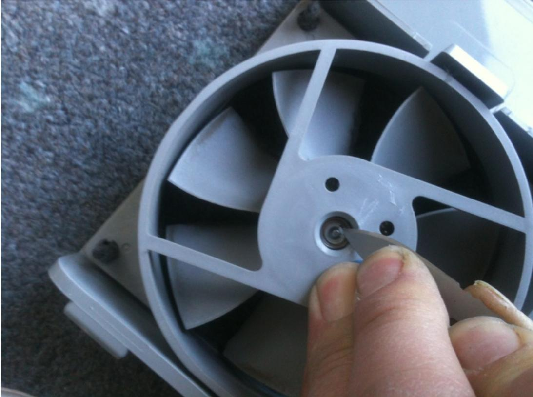
5. Shown below - clip removed. Don't worry if it looks a little damaged. They are surprisingly hard to destroy and, if you do manage to break it, you get a second chance later to keep the Zalman one undamaged.
