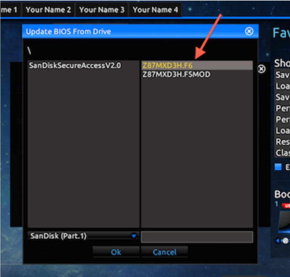
**CAUTION: DO NOT POWER DOWN OR INTERRUPT THE FLASHING PROCESS ONCE IT HAS STARTED. DOING SO COULD MAKE YOUR MOTHERBOARD COMPLETELY UN-USABLE. LET THE PROCESS COMPLETE ON IT'S OWN**
