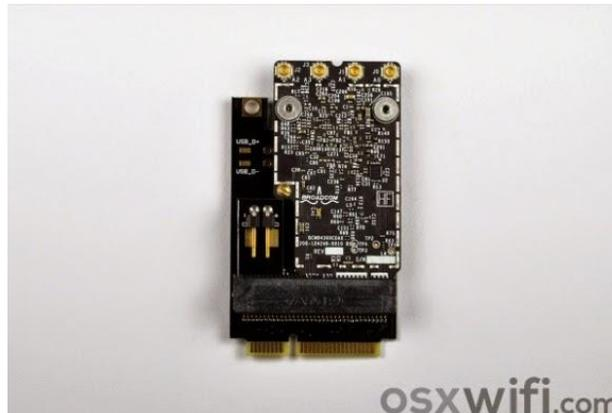
The first thing to note on these photos from the vendors website are that the card has 4 antenna connectors labeled J0 - J3. Note that [J2 is the Bluetooth antenna connector](#). If you are replacing an existing WiFi, it probably has just two connectors with a separate Bluetooth antenna connecting to the separate BT card. Never fear, Apple shipped the 2008 model Pro with all the antenna you will need, more on this when we get into the interior of the Mac.
